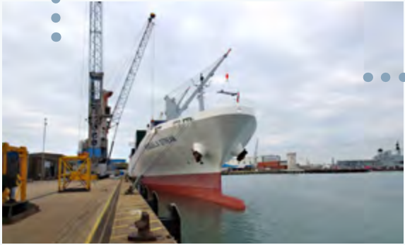
M.v. Benguela Stream featuring a bulb typical for Japanese-built reefers, optimized for a full cargo, the so-called 'banana draft'.
