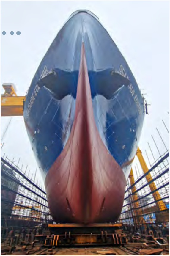
M.v. Seatrade Ecuador featuring a straight bow with a small bulb-shaped lower section.
