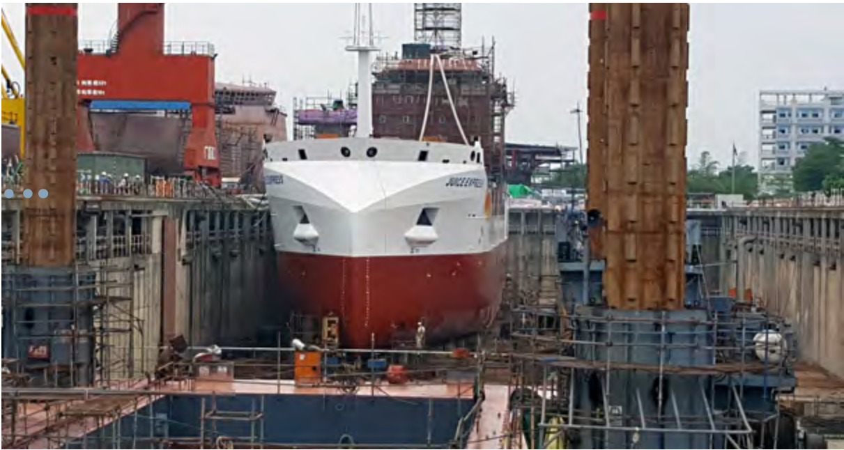
M.v. Juice Express featuring a straight bow with no bulb.
