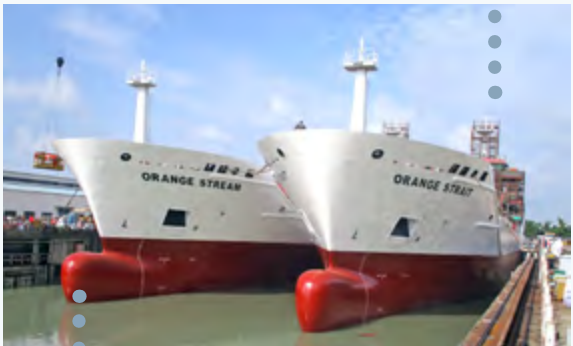
M.v. Orange Stream and m.v. Orange Strait featuring a full bulb designed by Marin Wageningen for these relatively slow and wide-beam vessels.
