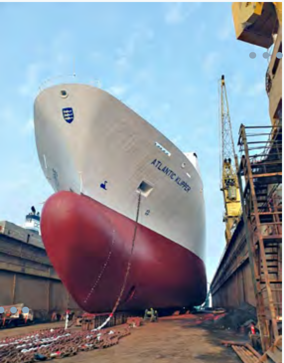
M.v. Atlantic Klipper featuring a heart-shaped bulb, slender at ballast draft and more balloon-like at summer draft. Also notice the previous owners' Jaczon Scheveningen bow shield and the 'ice knife', a vertical steel plate between the bulb and bow as part of this vessel's ice-class design.
