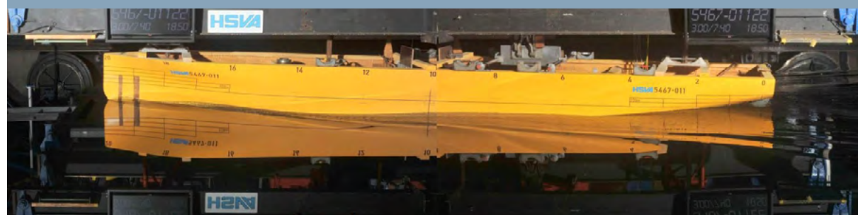
Steel cutting ceremony of Seatrade Chile ▲ 3D Tribon model of 1800 TEU reefer container vessel Seatrade Chile ► Model test at sea trial condition and speed of 18.5 knots ▼
